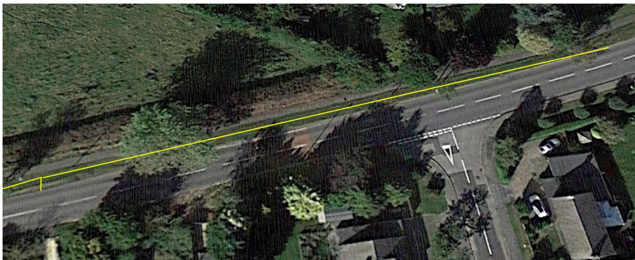
Figure 10: 2.4m x 100m visibility splay to the left for vehicles emerging from a West Road
